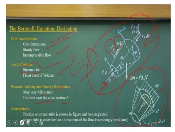
Now, let us have a the flow classifications or the simplifications that in this case we have considered one dimensional steady incompressible or compressible that is what we will discuss just a bit here. We have a stream tube, fixed control volume, okay. So, basically, as I told earlier, we have considering a stream tube concept, okay. That means for a steady flow, we have a series of this streamlines are there, defining their space along the stream tube.
