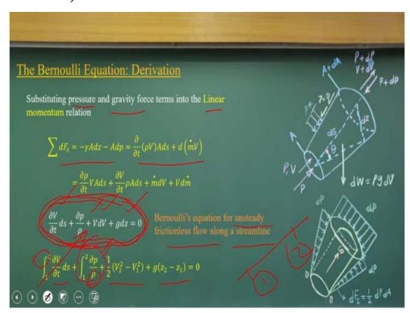
Now I am applying the linear momentum equations in streamline directions or streamwise directions. So sum of the force should be equal to the rate of change of the momentum in the control volume. Influx and the outflux, the momentum flux, the net what we will get at this part and this integrals we can simplify it into the part.
