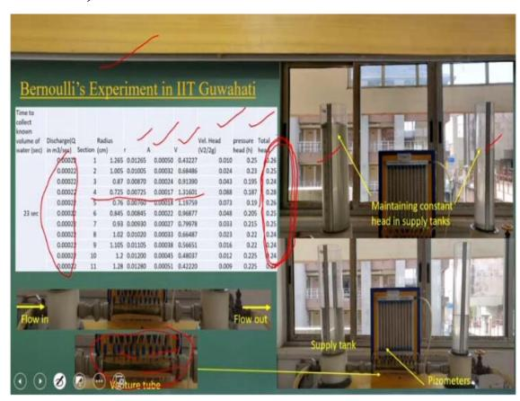
This is what the verification of Bernoulli equations in fluid mechanics lab in IIT, Guwahati. If you look at these ones, it has two tubes to maintaining the contents in supply heads. There is two tanks are there, which is maintaining the supply heads and here, you have a venture meters. We can very clearly look it, the cross sections area is decreasing it after certain times, again the cross section area is increasing.
